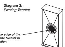
Push gently at the edge of the tweeter to point the tweeter in the desired direction.
